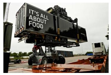
instead of roads is a new invention by TXLogistik, which makes it possible to lift regular cooling containers on to a train and back on a truck after transporting. This has not previously been possible.
